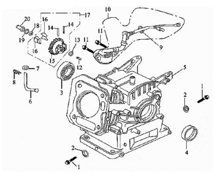
Note: When ordering parts from this list, specify: **Parts List A**, CRANKCASE ASSEMBLY and the ITEM No.
